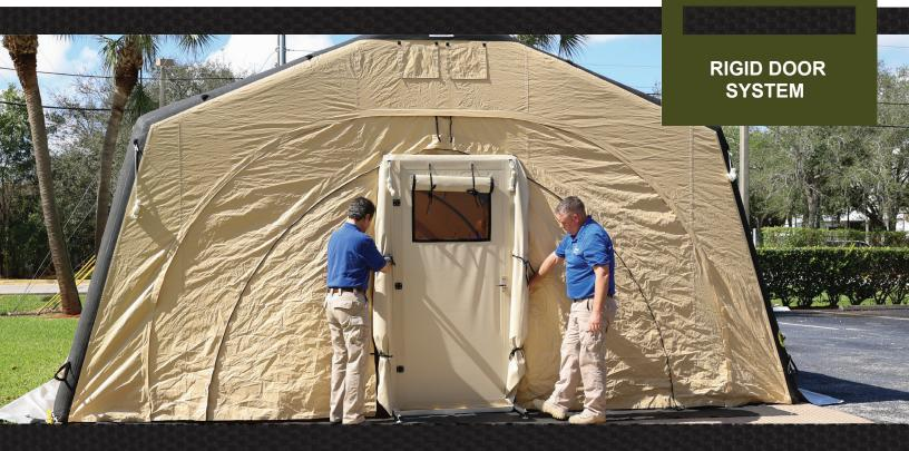
A rigid door option may be zippered into any ZUMRO shelter, in place of the roll-up man-doors. This option is especially useful during longer term deployments, where a conventional door is more desirable and efficient for shelter access than the roll-up configuration. Rigid door installation is easily accomplished by unzipping and removing the shelter connector panel, and zipping the attached rigid door panel into its place.
