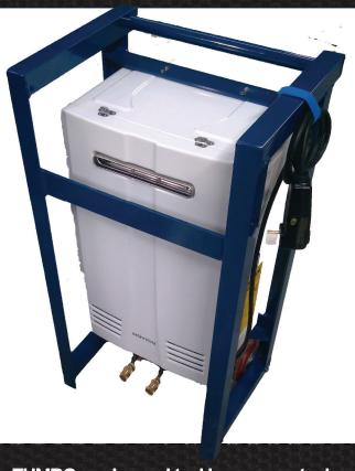
ZUMRO on-demand tankless gas water heaters provide a continuous supply of hot water; only heating the water needed. This unit is 80-83% efficient. The compact design of the ZUMRO 9952 tankless gas water heater delivers 5.8 GPM at a 54-degree F rise.
