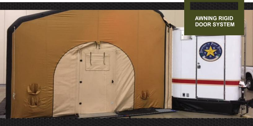
A rigid door option may be zippered into the ZUMRO Awning shelter, in place of the roll-up man-doors. This option is especially useful during longer term deployments, where a conventional door is more desirable and efficient for shelter access than the roll-up configuration. Rigid door installation is easily accomplished by unzipping and removing the shelter connector panel, and zipping the attached rigid door panel into its place.
