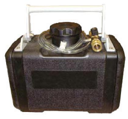
The ZUMRO Adjustable Soap Injector provides a simple way to inject soap directly in line during the decontamination process. Inductor is connected to inline water source. Once connected, set the needle to desired soap consistency depending on your protocol. The kit works well with the ZUMRO decon shower system and operates with water flows between 1 and 8 gpm.
