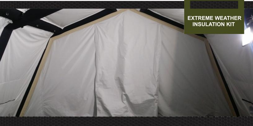
The Extreme Weather Insulation Kit features removeable vinyl-backed radiant barrier panels placed on the interior side of the air frame on all roof and sidewall panels. The lightweight panels offer both UV protection and a pocket of air insulation, which dramatically increases environmental control efficiency in hot and cold environments. The panels are pre-installed and deploy with the shelter.
