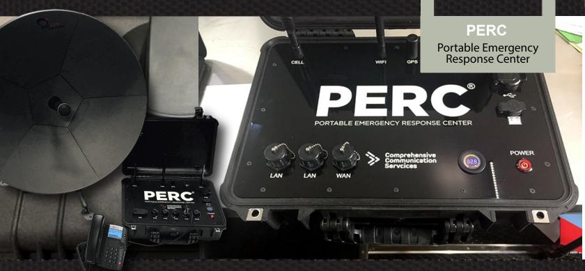
Simply press the power button, raise the LTE and Wi-Fi antennas or point the BGAN or VSAT antenna towards the southwestern skyline for satellite connectivity. In less than five minutes the PERC will connect to available cellular networks, a predetermined satellite and (optionally) local radios to establish a low cost wireless communication center for any approved, in-range devices.
