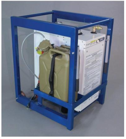
ZUMRO Part # 8907 Diesel Water Heater combines instant, continuouson-site water heating capabilities with compact size and sleek design. Mounted in an all aluminum welded frame with wheels and collapsible handles, the portable diesel water heater is easily transported anywhere on the emergency scene. An adjustable thermostat allows temperature adjustment during use. A 5 gallon buffered heat exchanger allows for minimal temperature fluctuation.
